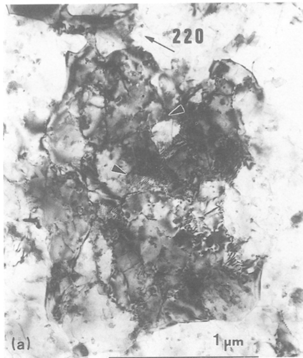
Figure 3 TEM images of a specimen deformed at 475°C, 10 MPa, for 2.7 \times 10^6 sec to a strain of 0.03. Grain morphology shows platelet shaped cluster of subgrains with low-angle boundaries (arrows). (a) Bright-field image with 001 pole parallel to beam, rolling plane parallel to page. (b) Dark-field image (111 spot) with rolling plane perpendicular to page, particles pin subgrain boundaries. Dislocation density in middle grain was greater than 4 \times 10^{13} \text{ m}^{-2} .
